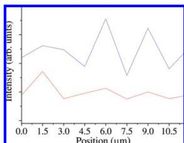
**Figure 5.** Line map of the molecularly imprinted polymer (MIP) droplet, displaying the intensities of the  $\sim 1385$  and  $\sim 1585 \text{ cm}^{-1}$  bands, shown in red and blue, respectively.
