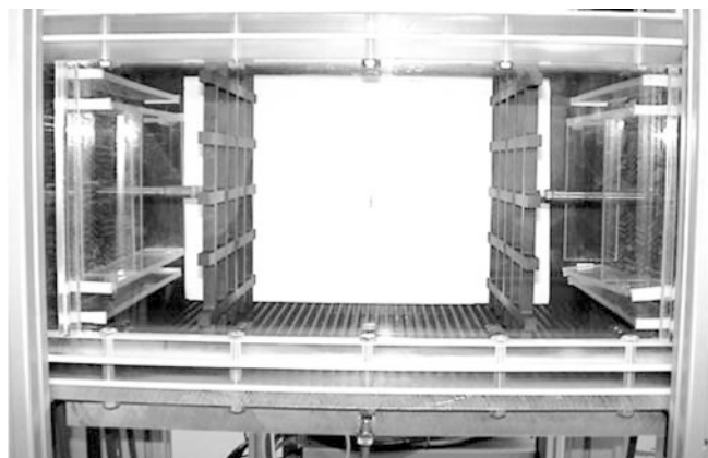
Fig. 2. The test section of the oscillating grids turbulence
