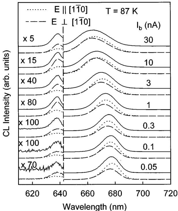
FIG. 2. Stack plots of normalized spatially integrated nonpolarized (solid line) and polarized (dashed lines) CL spectra taken for different probe currents at  $T=87 \text{ K}$ .
