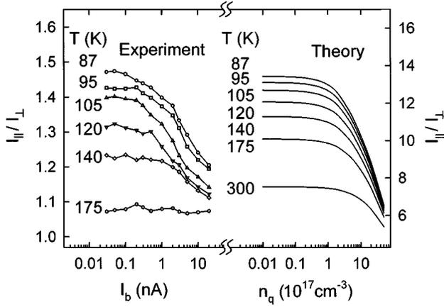
FIG. 4. Experimental and theoretical polarization ratios,  $I_{||}/I_{\perp}$ , as a function of the excitation density. Parallel and perpendicular subscripts are defined with respect to the  $[1\bar{1}0]$  quantum wire direction.
