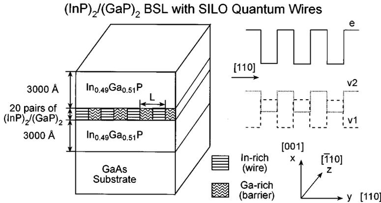
FIG. 1. A schematic diagram of the  $(\text{InP})_2/(\text{GaP})_2$  BSL and type-I to type-II superlattice modulation for  $e$ - $v1$  and  $e$ - $v2$  transitions.
