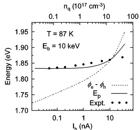
FIG. 3. Experimental and calculated energies of the peak CL intensity position,  $E_p$ , and calculated quasi-Fermi-level difference vs the excitation density and probe current.
