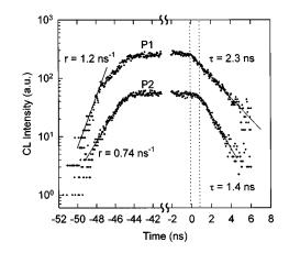
FIG. 3. CL transients including the onset and decay of the 410 nm luminescence taken near an exciton localization center (P1) and dark boundary region (P2).
