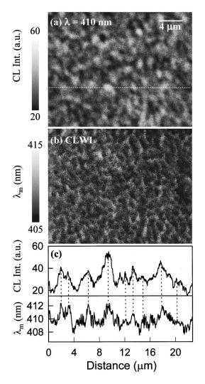
FIG. 2. (a) Monochromatic CL image, (b) CLWI image, and (c) line scan analysis for an e-beam current of 1 nA. The gray-scale bar serves as a key for the wavelength mapping in (b). The CL intensity of the scan at 410 nm and the peak wavelength,  $\lambda_m$ , along the dashed line in (a) are shown in (c).
