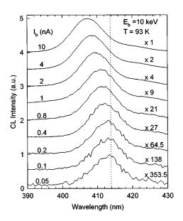
FIG. 1. Stack plots of normalized CL spectra taken with various probe currents.
