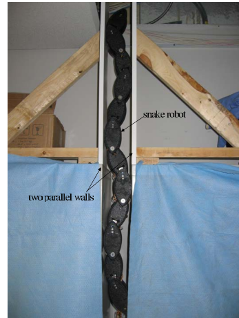
Fig. 1. Our newly developed snake robot climbing between two walls
