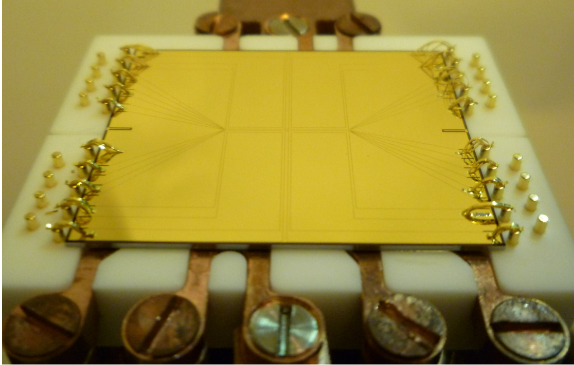
Figure 3.9: The atom chip on its mount: The chip is glued to the MACOR block that also holds the copper structure. The ribbon bonding between the chip and pins is visible at both edges of the chip, and the connection of the copper structure to the leads is visible at the top and bottom.
