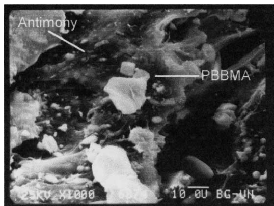
Fig 6. Scanning electron micrograph of sample 2. White PBBMA particle is identified in the micrograph. Small antimony particles are also indicated.
