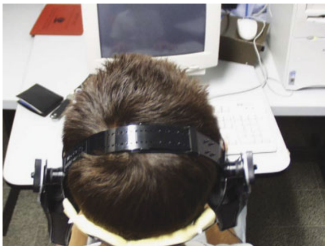
Fig. 5. A subject during the experiment, with the phone frame attached. [The color figure for this article is available online at www.interscience.wiley.com .]
